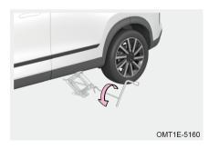
Step 3: Make sure all persons around the vehicle stay in the safe area, fit jack rocker into jack, and wheel bolt wrench into jack rocker, and turn wheel bolt wrench counterclockwise to lower the vehicle;
