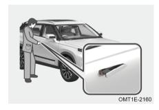
Step 2: Pull the door handle, insert the mechanical key into the keyhole inside the door handle, turn clockwise to unlock the door, counterclockwise to lock the door.
