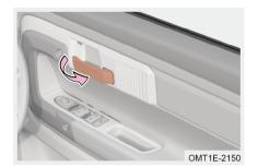
When doors are unlocked, pull door inside handle simply to open door. When doors are locked, pull door inside handle for the first time to unlock the door, and pull it again to open the door.
