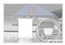
After SLA detects speed limit sign information on road in front and combines the information with speed limit information of navigation system, " indicator in instrument cluster remains on, if the speed exceeds current speed limit, it will have sound prompt or visual warning.
