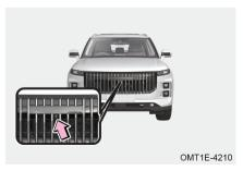
Installation position of front camera: located at intake grille of front bumper.
