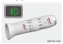
Turn vehicle power to ON mode, when position lights turn on, operate fog light switch to "  $\mbox{10}$ " position to turn on front fog lights; Turn vehicle power to OFF mode or operate fog light switch to "OFF" position again, front fog lights turn off.
