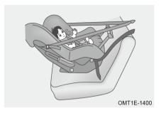
vehicle. Only install a rearward facing child restraint on the front passenger seat if the airbag is OFF. It is recommended children use a rearward facing child restraint system up to 4 years old.
