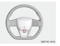
To sound the horn, press area near horn mark on the steering wheel.
