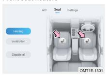
Method 1: After starting the vehicle, click front seat heater button by air conditioning display screen - seat - heating, it is 3-level heating (3 indicators on). Each time the switch is clicked, the heating level is lowered one level. Click it the fourth time to turn off the seat heating.
