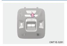
Manual activation: When required to report a serious accident, or require emergency help, long press the SOS button for 2 seconds.
