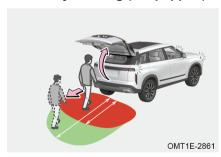
While vehicle power is switched to OFF mode or vehicle is started remotely, four doors are closed, approach to the back (red area) of vehicle when carrying smart key on your person and wait 3 seconds, after directional indicator lights come on, take a step back (green area), power boot door opens.
