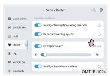
Overspeed alarm function can be turned on or off in the vehicle centre of the audio system.
