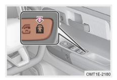
Press the switch, the switch indicator is on, and child-protector lock is locked. At this time, the rear door cannot be opened from inside the vehicle, but only from outside the car.
