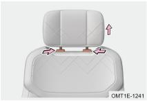
Removing head restraints: Pull the head restraint up completely while pressing 2 lock release buttons.
