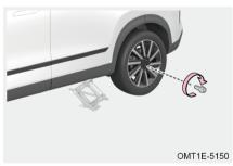
Step 2: When installing wheel bolts, screw into all wheel bolts clockwise by hand. Then straighten the spare tyre, and pretighten all wheel bolts with wheel bolt wrench;
