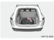
Step 2: Rotate fixing device of spare tyre counterclockwise to remove it, and then take out spare tyre.
