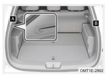
Pull the luggage curtain to the slots of point A and point B to secure it, and confirm if it is secured properly.
