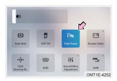
Turn vehicle power to ON mode, slide down from the top right edge of the audio system screen, click parking radar button, parking radar system turns on; when shift lever is not in R, click parking radar button again to exit.
