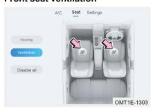
After starting the vehicle, click seat ventilation button by air conditioning display screen - seat - ventilate, it is 3-level ventilation (3 indicators come on). Each time the switch is clicked, the ventilation level is reduced by one level; Click it for the fourth time to turn off the seat ventilation.
