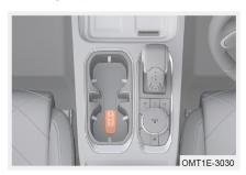
Step 1: Lay smart key onto the key marking of auxiliary fascia console cup holder (as shown in figure) with front side facing up; do not depress brake pedal at this time;
