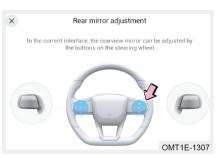
Turn vehicle power to ON mode, Audio System - Vehicle Centre -Vehicle comfort - Rear mirror adjustment.
