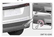
Step 1: Use a screwdriver with its tip taped to remove the rear towing eyelet hole cover.
