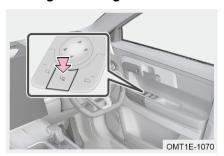
Operate using switch: When vehicle power is turned to ON mode, press outside rear view mirror folding switch to fold mirrors automatically, press the switch again to extend mirrors automatically.
