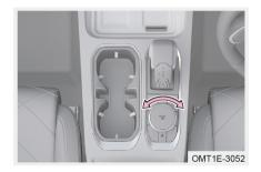
Rotate driving mode knob or set driving mode in unit head, the corresponding mode icon on instrument cluster will comes on accompanied by voice reminder to prompt you that driving mode is switched successfully.
