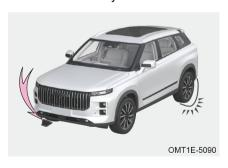
Step 1: Put a block under the tyre diagonally opposite to flat tyre to prevent vehicle from rolling.
