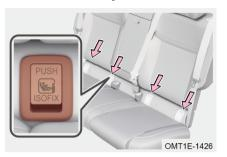
The rear outside seats are equipped with ISOFIX / i-Size anchorages. The anchorage locations are identified by a marking (see illustration) located on the seat back, directly above the associated anchorages. Please press the PUSH position to access the anchorages.
