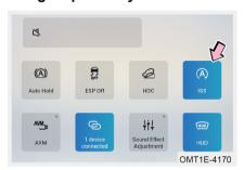
Turn vehicle power to ON mode, slide down from the top right edge of the audio system screen, click idling stop-start switch, idling stop-start system turns off; click idling stop-start switch again, idling stop-start system turns on.
