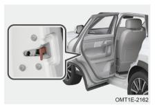
Vehicle cannot be locked electrically when battery is depleted or under similar conditions, in this case, the doors can be locked with emergency locking function.
