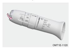
Turn vehicle power to ON mode, pull wiper combination switch towards the steering wheel and hold, the front washer sprays water, and front wiper operates simultaneously. Front washer will stop operating when the switch is released, the wiper will wipe 3 cycles at low speed, and operate one cycle then stop after a few seconds.
