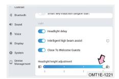
Turn vehicle power to ON mode, headlight height can be adjusted in the vehicle centre of the audio system
