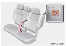
Adjust height of seat head restraints, remove them if necessary and fold up centre armrest. Then pull the left seatback adjustment handle forward and pull seatback forward to fold it down slowly. This can enlarge the luggage storage space.
