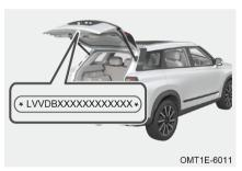
Vehicle Identification Number (VIN) label is located on boot door as shown in the illustration.
