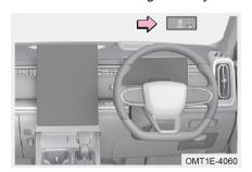
When head up display is turned on, a virtual image is formed in front of driver's field of vision to display the corresponding vehicle speed, driving mileage and other information.
