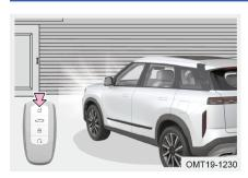
Turn the headlight combination switch to "AUTO" position before stopping. When the vehicle is in a dim environment, press unlock button on smart key, the low beam lights come on for 27 seconds.
