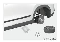
Step 5: Remove the wheel bolts of flat tyre counterclockwise with the wheel bolt wrench, and remove the flat tyre.
