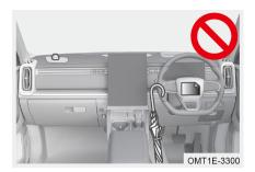
Do not attach anything to or lean anything against the areas such as the instrument panel, steering wheel and lower portion of the instrument panel. These items can become projectiles when driver airbag or front passenger airbag deploys.
