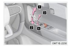
Operate power window switch after vehicle power is switched to ON mode:
