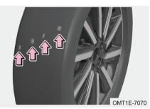
Check the tyre tread by tread wear mark. When tread wear reaches its limit, tread will be in the same plane as the wear band. If such condition occurs, the tyre performance and safety will be seriously impacted, and replacement is necessary.
