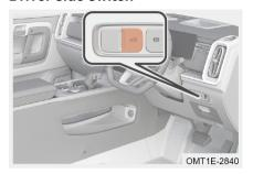
With central control lock unlocked, long press " " switch, directional indicator lights will come on and power boot door will be opened/ closed.
