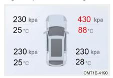
When tyre temperature is higher than 85° C and speed is no less than 15 mph (25 km/h) for a period of time, system will send a high temperature warning, corresponding wheel symbol will blink, current tyre temperature value will be displayed and " !! " yellow indicator in instrument cluster will remain on.
