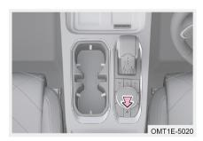
In case of vehicle failure or traffic accident etc., please turn on the hazard lights to warn other vehicles, so as to avoid the secondary accident.
