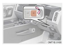
When vehicle power is switched to ON mode, or engine starts and vehicle is stopping, pull up the electric parking brake button, " (P)" red indicator in instrument cluster and electric parking brake button indicator remains on, indicating parking brake function has been turned on.
