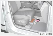
Vehicle Identification Number (VIN) is stamped under driver's seat.
