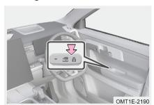
Press passenger side window OFF switch, passenger side window OFF switch indicator comes on, passenger side window switch will be disabled. After disabling, only window switches on driver side can be used to operate passenger side windows (this function is recommended when there is a child in vehicle). Press the switch again to cancel this function and the indicator goes off.
