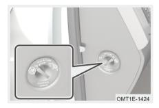
The airbag enabling/disabling switch is located on the passenger side instrument panel and is visible when front passenger door is opened.
