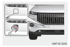
Step 1: Use a screwdriver with its tip taped to remove the front towing eyelet hole cover;
