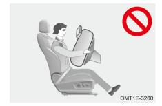
Alwavs keep SRS airbag deployment path clear. lt is forbidden to place anything (such as mobile phone) between the occupant and the SRS airbag and fix or place any objects on or near the SRS airbag cover: If there is an object between occupant and SRS airbag, the SRS airbag may not deploy according to design path, or the SRS airbag may push object to occupant's body, causing serious injury or even death.
