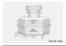
Brake fluid level should be between the "MIN" and "MAX" marks. If the level is at or below the "MIN" mark, add brake fluid and contact the authorized service centre for inspection and repair immediately.
