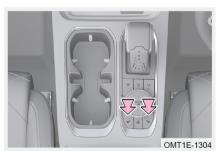
Method 2 (if equipped): After starting the vehicle, press the front seat heater switch on the auxiliary fascia console. it is 3-level heating (3 indicators on). Each time the switch is pressed, the heating level is reduced by one level. Press it the fourth time to turn off the seat heating.
