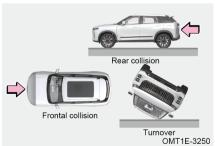
The side airbags, curtain shield airbags and front middle airbag may not deploy if the vehicle is subjected to a front or rear collision, turnover or low speed side collision.
