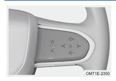
Customization button " \( \frac{1}{2} \) ": This button can be customized in audio system - Vehicle Centre - Vehicle Settings.
