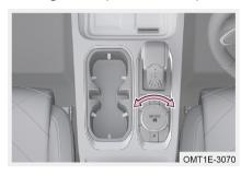
System is ECO mode by default when engine starts. Rotate driving mode knob between SPORT mode, ECO mode or NORMAL mode. You can choose according to different road conditions.
