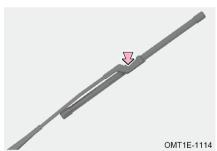
Step 1: Operate the front wiper switch within 3 seconds after turning off the engine start stop switch, the wiper will enter repair mode;
