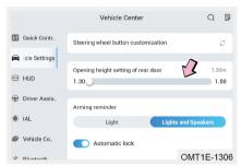
Method 2: Turn vehicle power to ON mode, set the opening height by Audio System - Vehicle Centre - Vehicle Settings.
