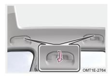
Assist grips are installed above front passenger door and both rear passenger doors respectively.
