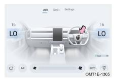
After starting the vehicle, press "" on the air conditioning system screen to turn on steering wheel heating function. After pressing the button again, steering wheel heating function is turned off.
