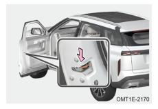
Open the door, move the button downward to lock door; Pull the door handle to make sure the door is locked.
