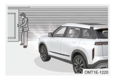
ON: Turn vehicle power to OFF mode. and turn the headlight combination switch "AUTO" to position. When the vehicle is in a dim environment, press lock button on smart kev. vehicle is locked successfully. Low beam lights automatically come on for 27 seconds. Press lock button on smart key to activate it again.
