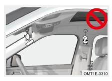
Do not attach anything to areas such as the door, windshield glass, side door glass, A pillar, B pillar, C pillar, roof side rail and assist grip.
