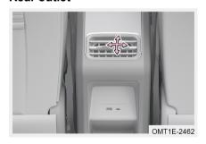
Move rear outlet adjustment lever up, down, left or right by hand to adjust direction of airflow.
