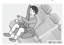
For larger children that cannot fit in a child restraint system with a high back, they may occupy a second row outboard seat using a booster seat. either attached to the lower anchorage points or belted, described in the instructions provided bv the child restraint system manufacturer.
