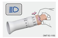
Turn vehicle power to ON mode, when turning on low beam lights, pull headlight combination switch away from steering wheel side and release, high beam lights remain on; Pull headlight combination switch towards steering wheel side and release to turn off high beam lights.
