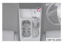
While vehicle power is switched to ON mode, the wireless charging starts to work after putting the mobile phone in wireless charging sensing area, and the audio head unit displays " (1)") ". The audio head unit displays " (1)") " after charging is completely.
