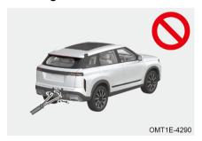
When washing vehicle, use a soft cloth or water (low water pressure) to wash off foreign matter such as snow, mud, and dust on the surface of the radar sensor.
