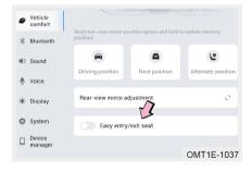
Turn vehicle power to ON mode, turn on easy entry / exit seat function by Audio System - Vehicle Centre - Vehicle comfort.
