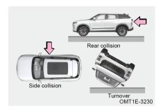
The driver airbag, front passenger airbag and driver knee airbag will usually not deploy if the vehicle is involved in a side or rear collision, if it rolls over, or if it is involved in a low-speed frontal collision.
