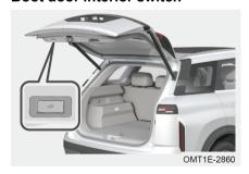
When the power boot door opens, press " " switch to close it
