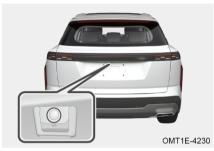
Installation position of rear camera: located on center part above rear license plate.
