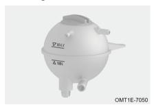
When engine is cold, the coolant level should be between the "MIN" and "MAX" marks. If the level is at or below the "MIN" mark, add coolant and contact the authorized service centre for inspection and repair immediately.
