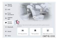
Turn vehicle power to ON mode, the audio system will pop up vehicle comfort screen, select driving position, rest position or alternate location, long press to update and memorize.
