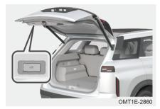
Method 1: When the power boot door is open, adjust it to your desire height; long press " " switch until the vehicle gives a light prompt, and the power boot door opening height is set successfully.
