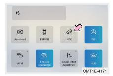
With vehicle power in ON mode, slide down from the top right edge of the audio system screen to display the shortcut menu screen.
