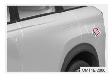
Step 1: After the vehicle is unlocked, push the fuel tank cover and it will pop up;
