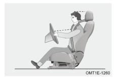
The shoulder belt should be over the centre of the shoulder and close to the chest, kept away from the neck, the lap belt should lie over the hips instead of stomach.
