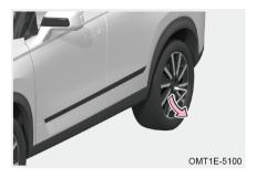
Step 2: Fit wheel bolt wrench to wheel bolt of flat tyre, set the handle on left side, hold the end of wrench handle and push it downward, loosen each bolt of flat tyre about one-half turn;
