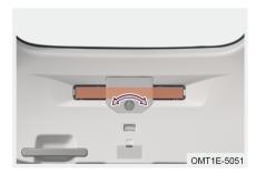
Warning triangle is located on the boot door panel, turn the retaining clamp counterclockwise to remove it
