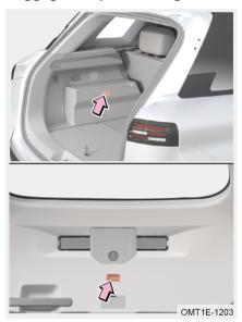
When boot door is opened, luggage compartment lights will turn on for several seconds automatically. When boot door is closed, luggage compartment lights will turn off immediately.
