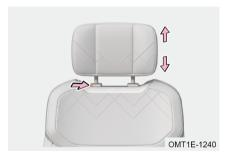
Adjust head restraint upward: Pull it up directly to a proper height.
