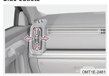
Move left/right side outlet adjustment lever up, down, left or right by hand to adjust direction of airflow.
